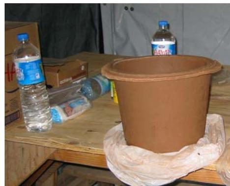
Place the pot in a dry area for a day or so. Avoid drying it too quickly or the pot will crack. Direct sunlight, especially in the hot summer months, should be avoided.
