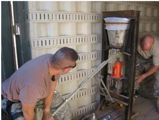
The mold is then closed by pumping the jack handle or operating the motor (depending on the type of press) until the male and female molds meet.
