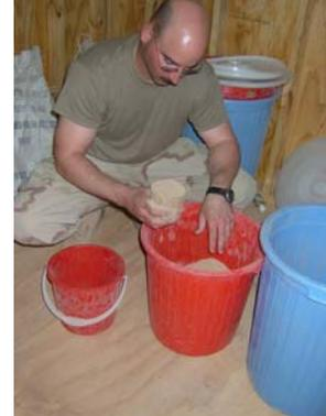
The mix proportions can be done using any scoop and varying the number of scoops for each of the ingredients. For example, a 60:40 mix can be obtained by using 3 scoops of clay to 2 scoops of friable material.
