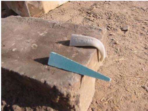
*Note: Measuring the temperature in the Kiln can be done with Pyrometric Cones which melt when they have been 'at temperature' for a certain amount of time. Such as those in our 55-gallon drum kiln. The cone is placed at sight level through the peep hole. When the temperature has been reached for the proper amount of time they will melt over (like the white cone on the left).*
