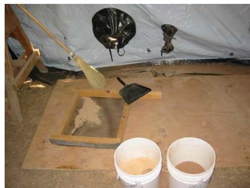
The same process is used for the friable material to ensure particle size consistency in the mix.
